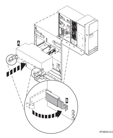
Figure 25. Install a power supply in a stand-alone model
