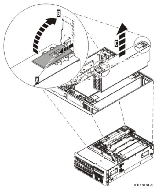
Figure 37. Remove a power supply from a rack-mounted system unit
