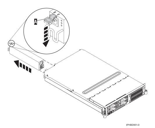
Figure 13. Remove a power supply
