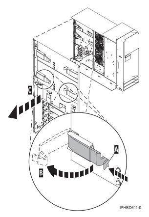
Figure 23. Remove a power supply from a stand-alone model
