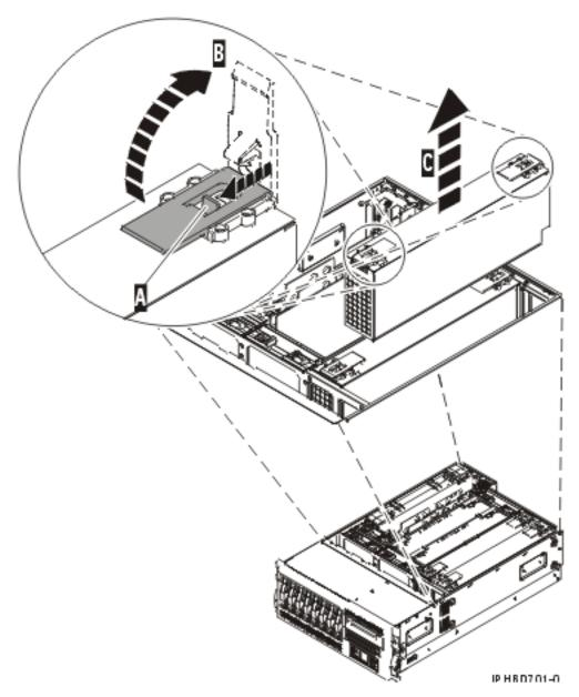
Figure 42. Remove a power supply from rack-mounted system unit
