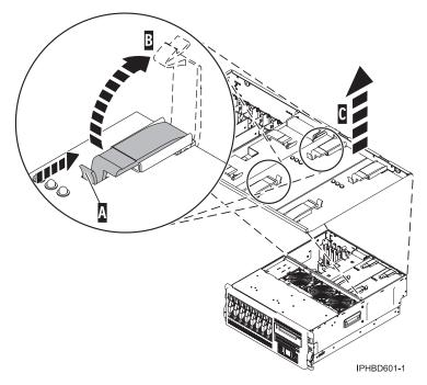
Figure 22. Remove a power supply from a rack-mounted model
