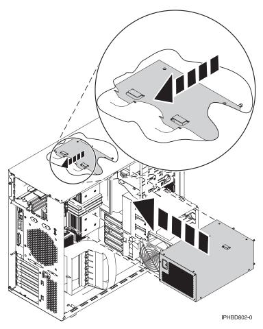
Figure 4. Attaching the power supply
