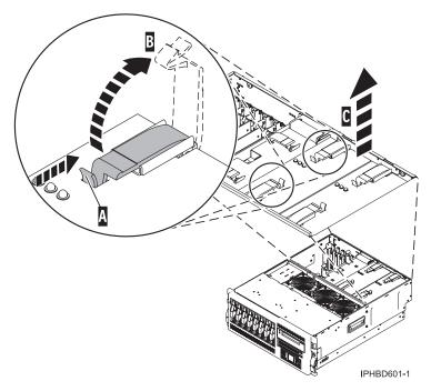
Figure 27. Power supply removal from a rack-mounted system unit
