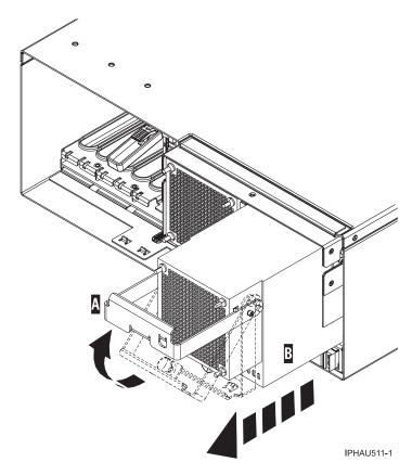
Figure 48. Remove the power supply from a system unit
