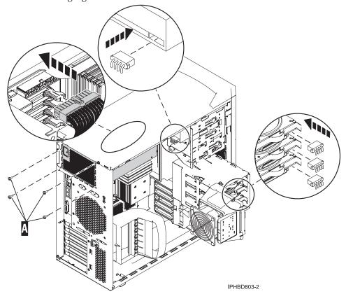
5. Attach the power connectors to the system in the locations you noted in the remove process.
