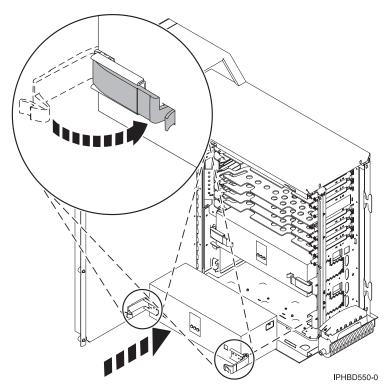
Figure 61. Power supply installation
