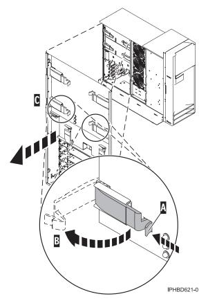
Figure 29. Power supply removal from a model 285 stand-alone system unit
