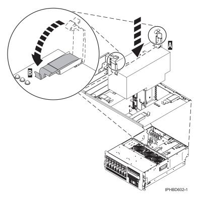
Figure 30. Replace a power supply in a rack-mounted system unit
