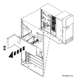
Figure 21. Remove a power supply filler
