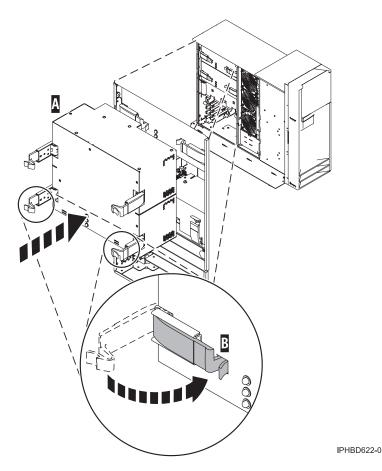
Figure 33. Replace a double wide power supply in a stand-alone system unit
