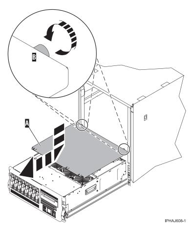
Figure 70. Install the service access cover on the rack-mounted model
