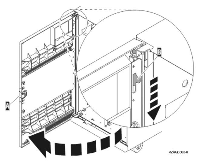
Figure 72. Removing the expansion unit front door
