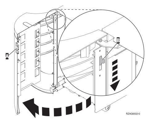
Figure 74. Removing the expansion unit back door
