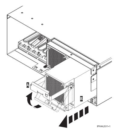
Figure 52. Remove the power supply
