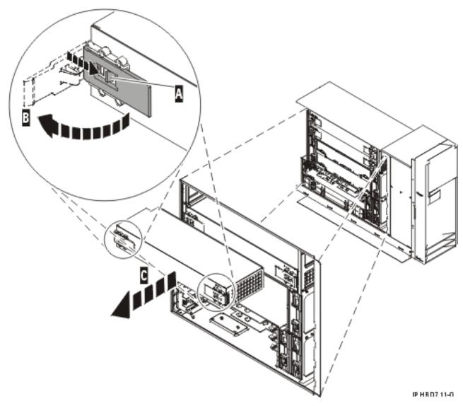
Figure 38. Remove a power supply from a stand-alone system unit
