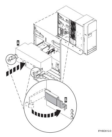
Figure 31. Replace a power supply in a stand-alone system unit
