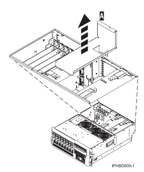
Figure 20. Remove a power supply filler t
