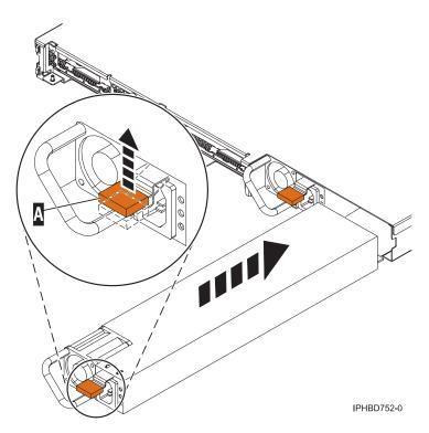
Figure 10. Install a power supply
