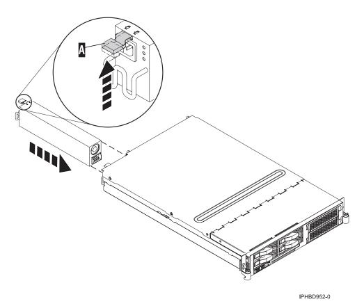
Figure 17. Install a power supply
