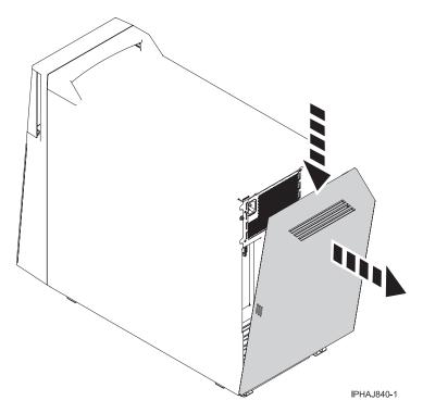
Figure 64. Removing the back cover
