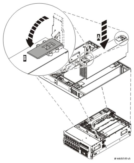
Figure 44. Replace a power supply in a rack-mounted system unit
