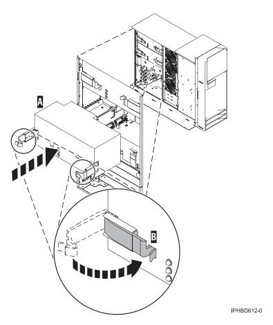
Figure 32. Replace a power supply in a model 285 stand-alone system unit
