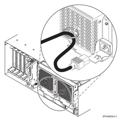
Figure 50. Cable routed through power supply ring
