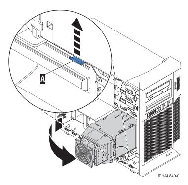
Figure 1. lifting the disk drive cage
