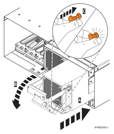
Figure 49. Replace the power supply
