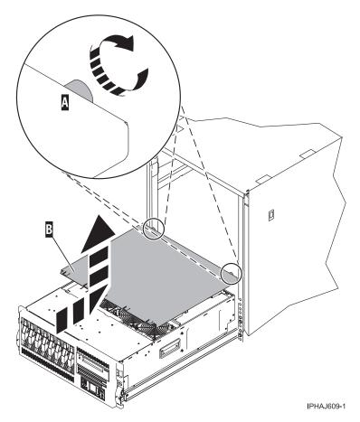
Figure 68. Remove the service access cover
