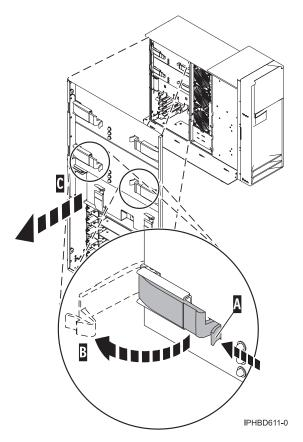
Figure 28. Power supply removal from a stand-alone system unit
