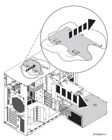
Figure 3. Detaching the power supply
