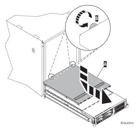
Figure 71. Install the service access cover on the rack-mounted model
