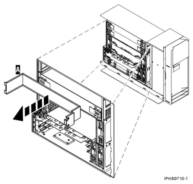
Figure 36. Remove a power supply filler from a stand-alone system unit
