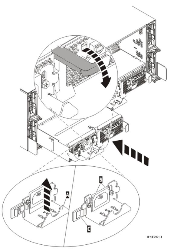
Figure 55. Power supply installation
