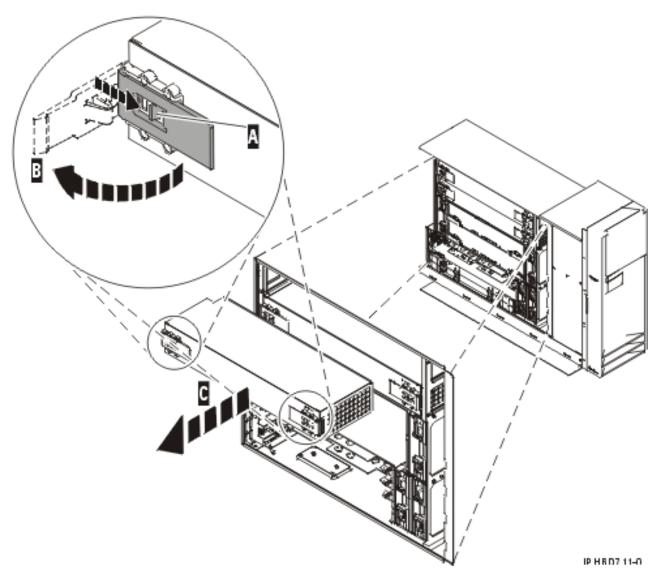
Figure 43. Remove a power supply from a stand-alone system unit
