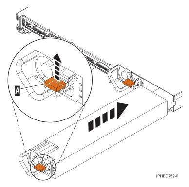
Figure 8. Install a power supply
