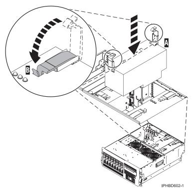
Figure 24. Install a power supply in a rack-mounted system model
