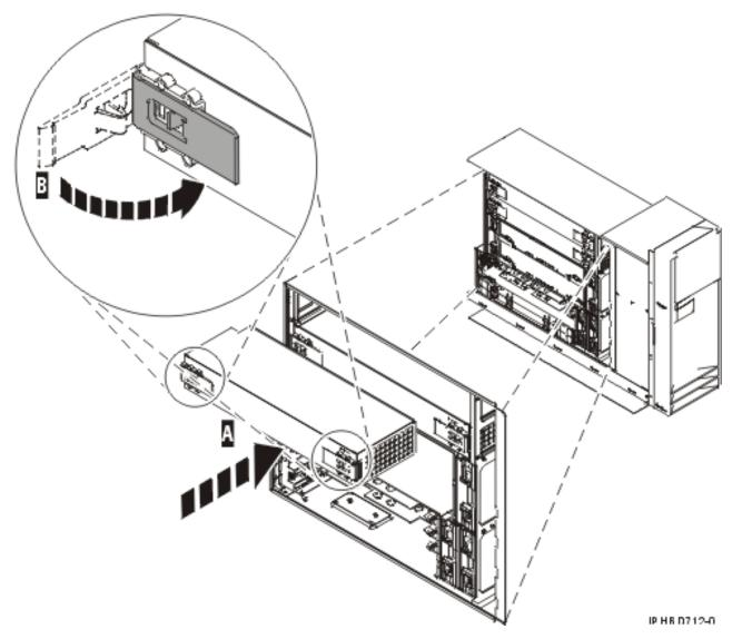
Figure 40. Install a power supply in a stand-alone system unit
