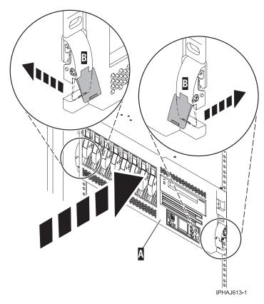
2. Replace and tighten the two thumbscrews B that secure the system or expansion unit A to the rack as shown in the following figure.
