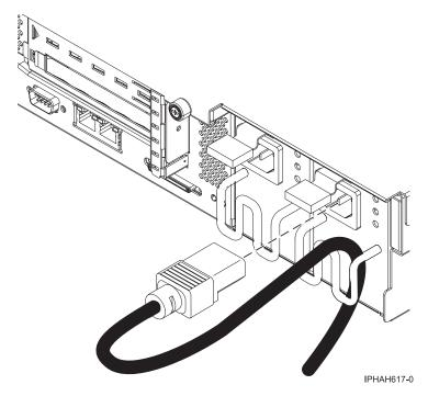
Figure 15. Route the power cable through the bar
