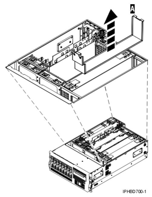
Figure 35. Remove a power supply filler from a rack-mounted system unit
