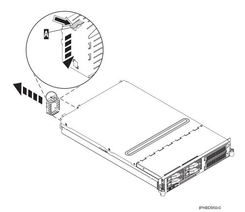
Figure 12. Remove a power supply filler
