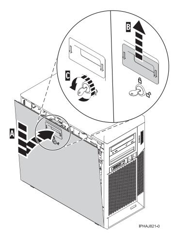
Figure 67. Replacing the service panel
