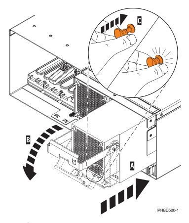
Figure 53. Replace a power supply
