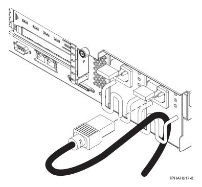
Figure 18. Route the power cable through the bar
