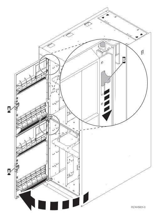
Figure 73. Removing the expansion unit front door
