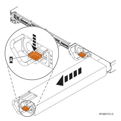
Figure 9. Remove a power supply
