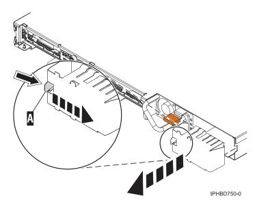
Figure 6. Remove a power supply filler
