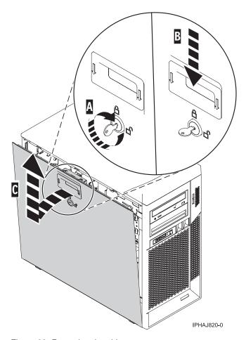
Figure 66. Removing the side cover
