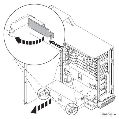
Figure 60. Power supply removal
