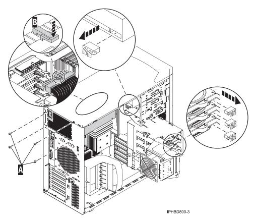
Figure 2. Removing the power supply connections
