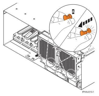
Figure 51. Power supply unlocked
