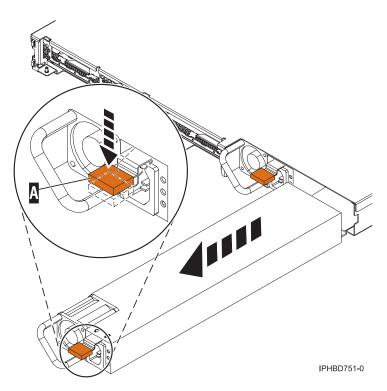
Figure 7. Remove a power supply
