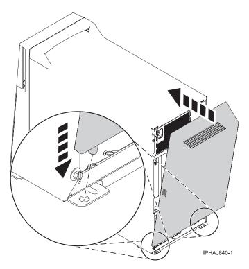
Figure 65. Replacing the back cover
