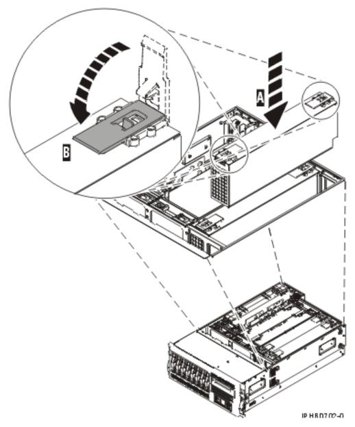
Figure 39. Install a power supply in a rack-mounted system unit
