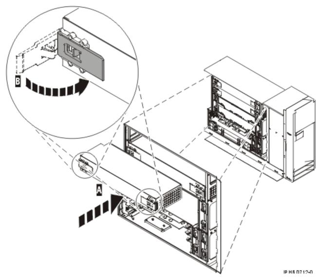
Figure 45. Replace a power supply in a stand-alone system unit
