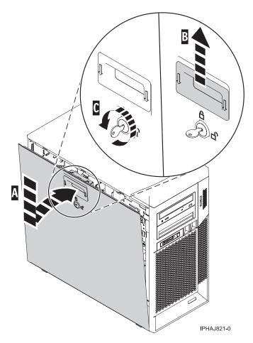
Figure 18. Replacing the service panel
