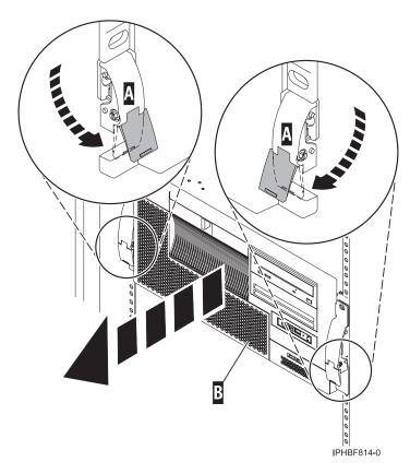
Figure 13. Placing the model in the service position
