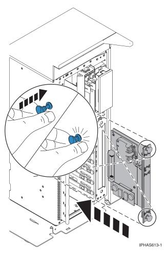
Figure 7. RAID enablement card replacement in a stand-alone system unit
