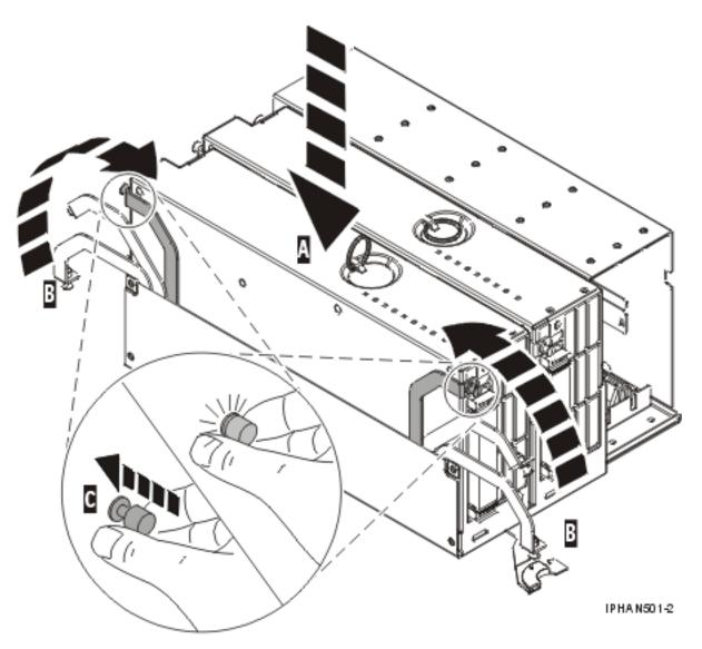
Figure 11. Replace the model 9116-561 or 570 backplane assembly
