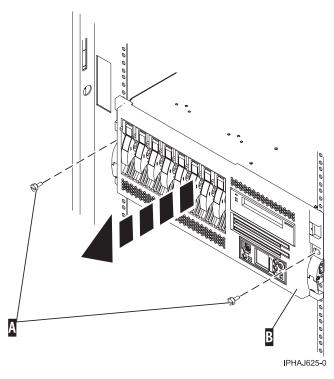
3. Release the rack latches A on both the left and right sides as shown in the following figure.
