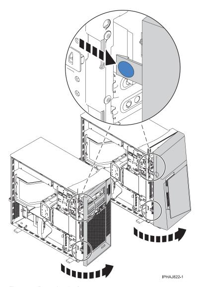
Figure 14. Removing the front cover
