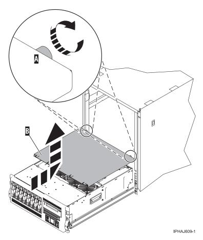
Figure 21. Remove the service access cover
