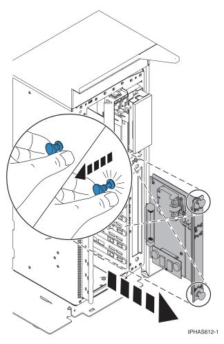
Figure 5. RAID enablement card removal from a stand-alone system unit
