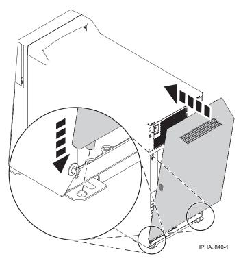
Figure 16. Replacing the back cover
