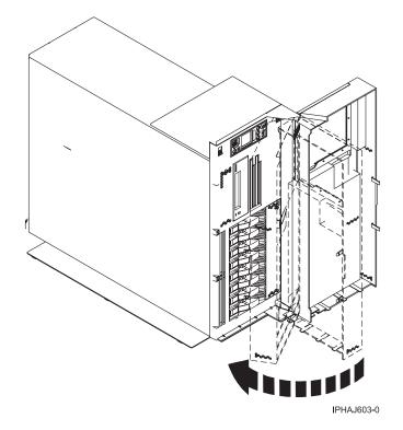
Install the door on the model 285 or 9131-52A:
