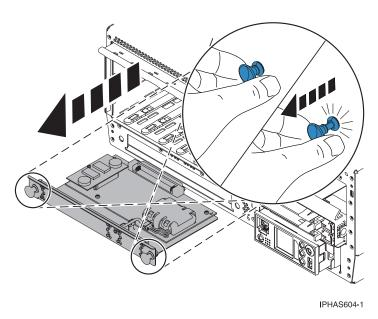
Figure 6. RAID enablement card removal from a rack-mounted system unit
