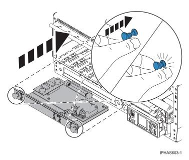
Figure 8. RAID enablement card replacement in a rack-mounted system unit
