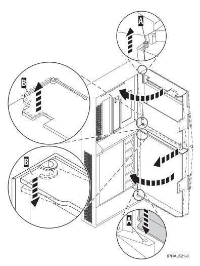
Figure 20. Installing the model 285 door
