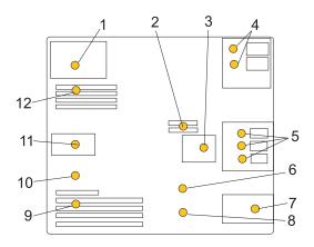
Figure 27. Light path diagnostic card indicator LED layout
