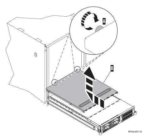
Figure 22. Remove the service access cover
