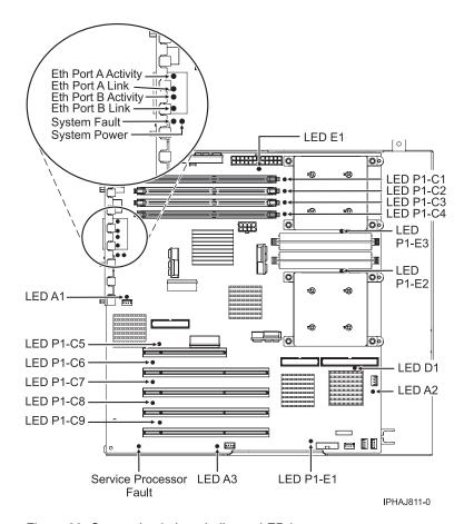
Figure 28. System backplane indicator LED layout
