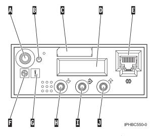
**Tip:** The system attention light G, as shown in the previous figure, does not appear on the control panel on the model 570.
