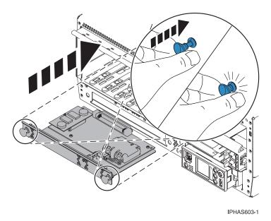
Figure 4. Rack-mounted system unit RAID enablement card replacement
