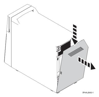
Figure 15. Removing the back cover
