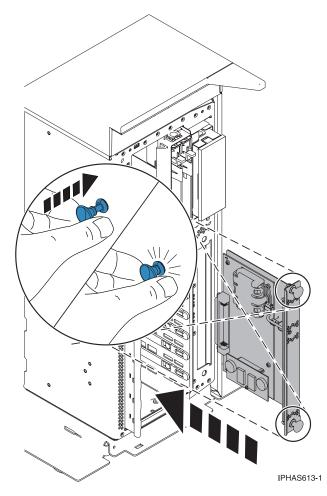
Figure 3. Stand-alone system unit RAID enablement card replacement
