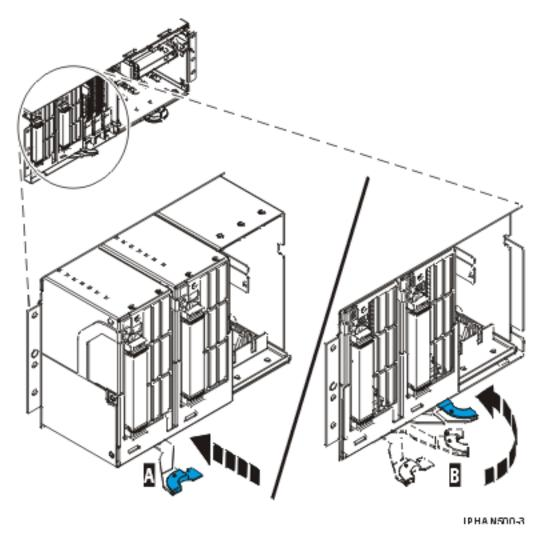
Figure 12. Slide the model 9116-561 or 570 system backplane assembly into the system unit
