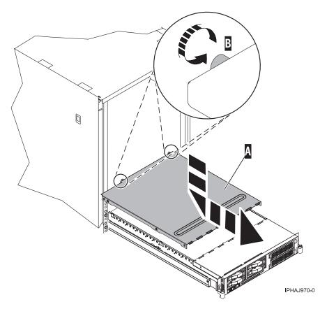
Figure 24. Install the service access cover on the rack-mounted model
