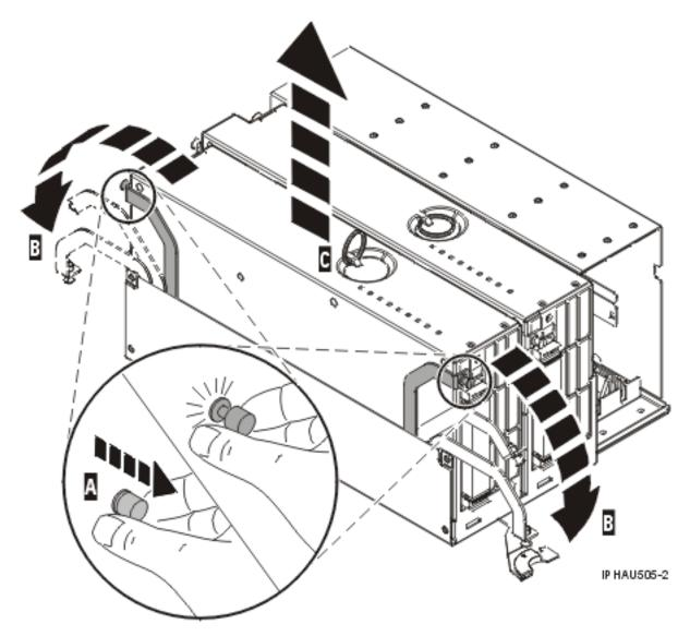
Figure 10. Remove the processor assembly from model 9116-561 or 570 backplane assembly
