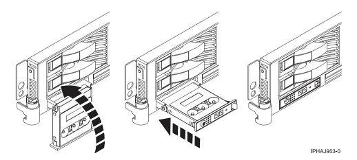
Figure 26. Close the control panels
