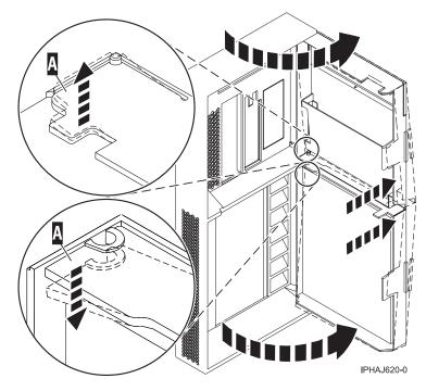
Figure 19. Removing the model 285 or 9131-52A door
