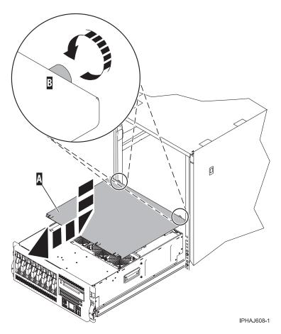
Figure 23. Install the service access cover on the rack-mounted model
