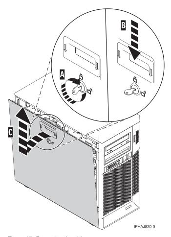
Figure 17. Removing the side cover
