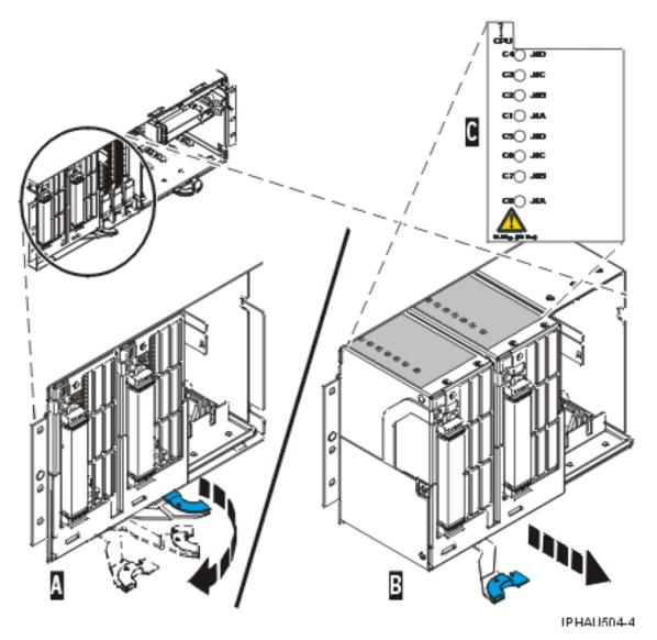
Figure 9. Slide the model 9116-561 or 570 system backplane assembly out of the system unit
