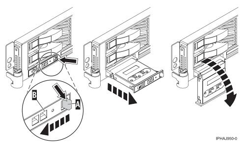
Figure 25. Gain access to the control panels
