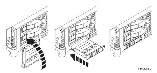
Figure 56. Close the control panels
