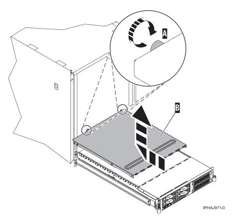
Figure 43. Remove the service access cover
