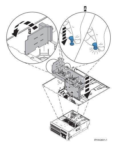
Figure 28. Replacing the model 52x fan tray assembly in a rack-mounted system
