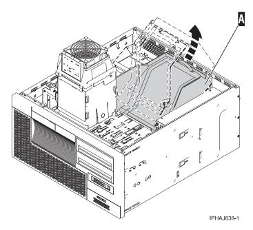
Figure 3. Removing the system unit air baffle in a rack-mounted system
