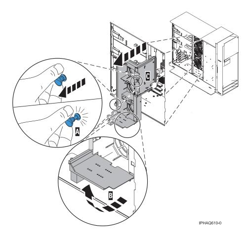
Figure 27. Removing the fan tray assembly from a stand-alone system
