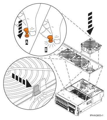
Figure 24. Replacing the model 52x system unit fan in a rack-mounted system
