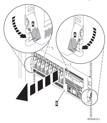
4. Review the following note, and then slowly pull the system or expansion unit out from the rack until the rails are fully extended and locked.
