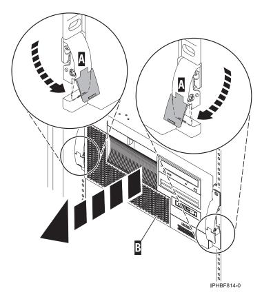
Figure 38. Placing the model in the service position
