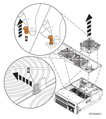
Figure 22. Removing the model 52x system unit fan in a rack-mounted system
