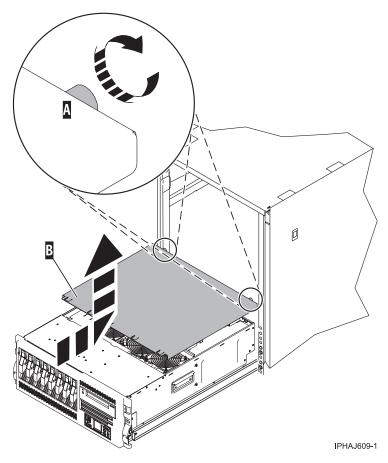
Figure 42. Remove the service access cover
