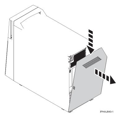
Figure 47. Removing the back cover
