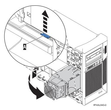
Figure 11. Lifting the disk drive cage
