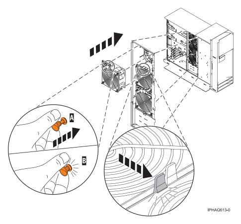
Figure 25. Replacing the model 52x or IntelliStation POWER 285 system unit fan in a stand-alone system
