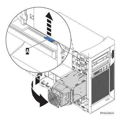
Figure 1. Open the disk drive cage
