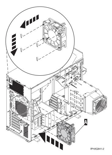
Figure 14. Replacing the system unit fan in a stand-alone system
