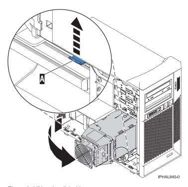
Figure 9. Lifting the disk drive cage
