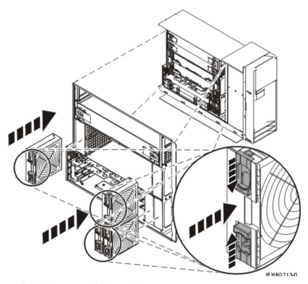
Figure 33. Replacing the system unit fan in a stand-alone system
