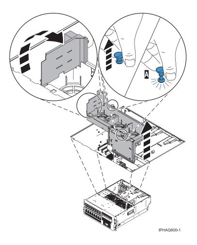
Figure 26. Removing the fan tray assembly in a rack-mounted system removal
