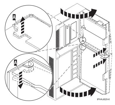
Figure 51. Removing the model 285 or 9131-52A door
