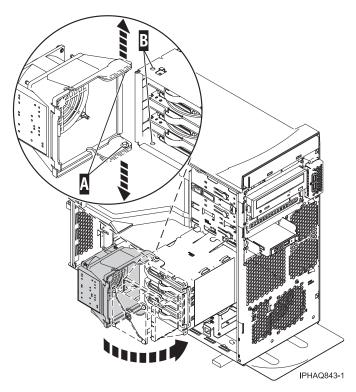
Figure 15. Attaching the disk drive cage fan
