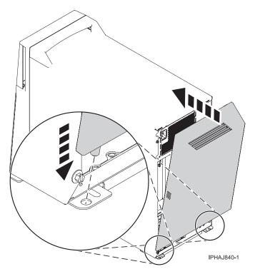
Figure 48. Replacing the back cover
