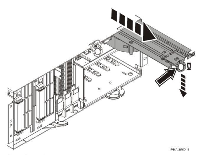
Figure 36. Fan removal
