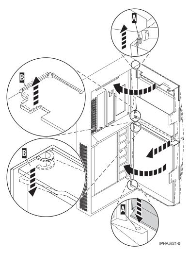
Figure 52. Installing the model 285 door
