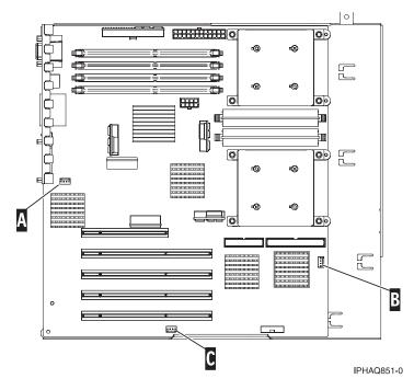
Figure 17. Fan power connector locations
