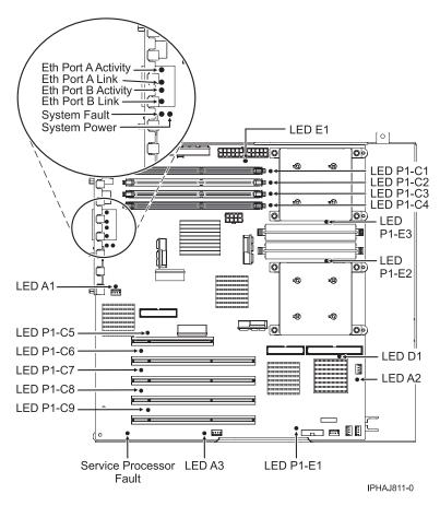
Figure 54. System backplane indicator LED layout
