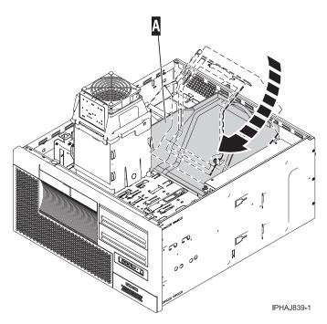
Figure 6. Replacing the model 7047-185 or 7037-A50 system unit air baffle in a rack mounted system.
