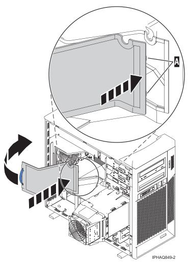
Figure 7. Attaching the air baffle door
