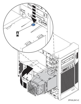
Figure 8. Closing the disk drive cage
