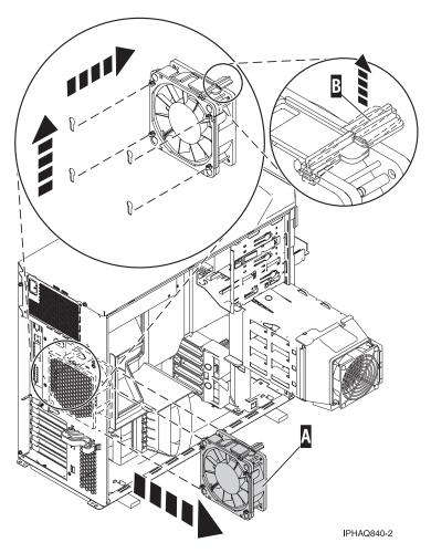
Figure 10. Removing the system unit fan in a stand-alone system
