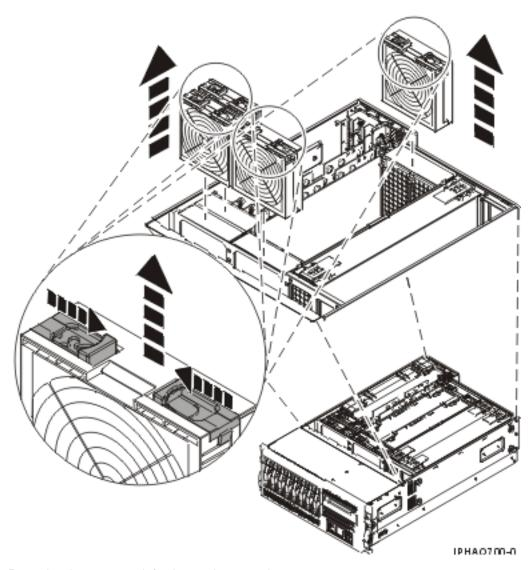
Figure 30. Removing the system unit fan in a rack-mounted system
