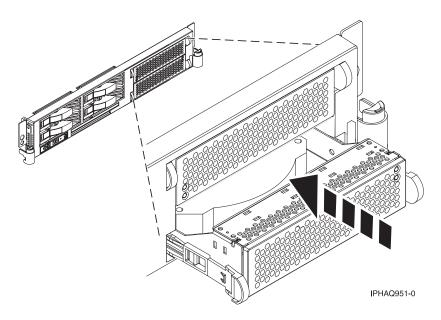
Figure 21. Rack-mounted system unit fan replacement
