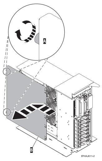
2. Slide the service access cover toward the back of the system unit. When the front of the cover clears the front frame ledge, lift the cover off the system unit.
