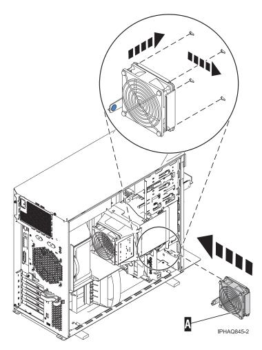
Figure 16. Installing the PCI adapter fan
