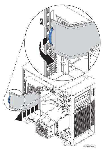
Figure 2. Removing the air baffle door
