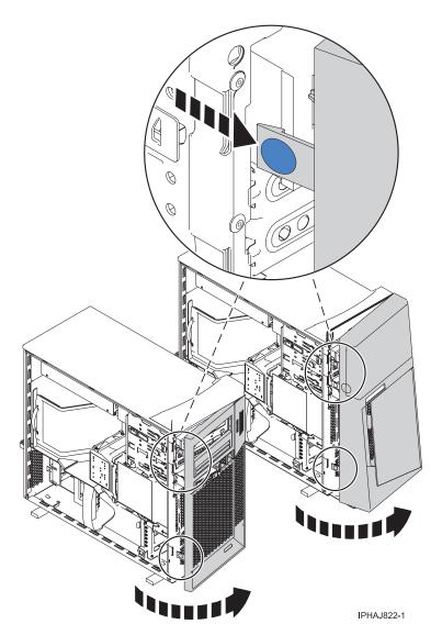
Figure 46. Removing the front cover
