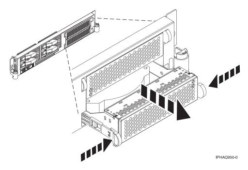
Figure 20. Rack-mounted system unit fan removal
