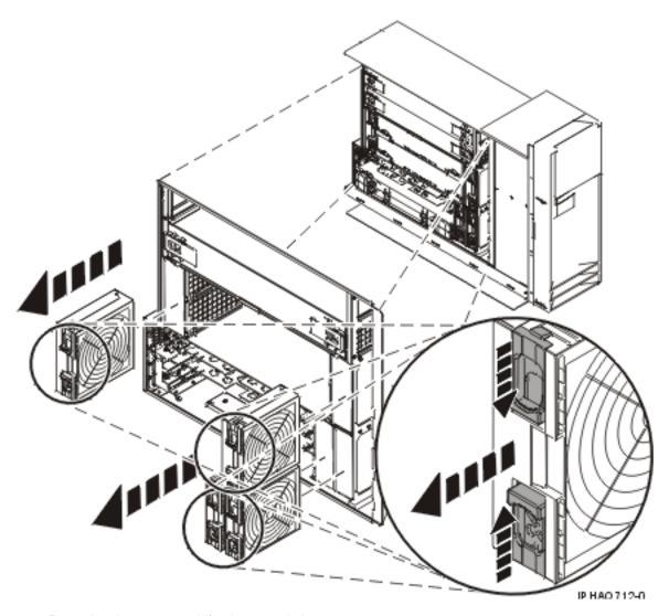
Figure 31. Removing the system unit fan in a stand-alone system
