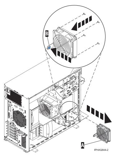
Figure 13. Removing the PCI adapter fan
