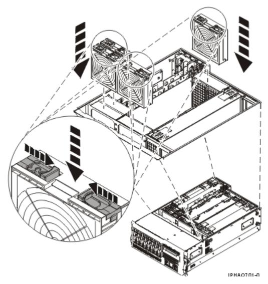
Figure 32. Replacing the system unit fan in a rack-mounted system
