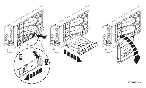
Figure 55. Gain access to the control panels
