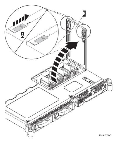
Figure 40. Open the service access panel
