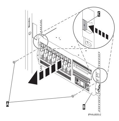
Remove the front cover from the stand-alone model 285, 52x, 55x, or OpenPower 720:
