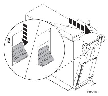
4. Gently pull the cover up and off the base, releasing the lower cover-locking tabs.
