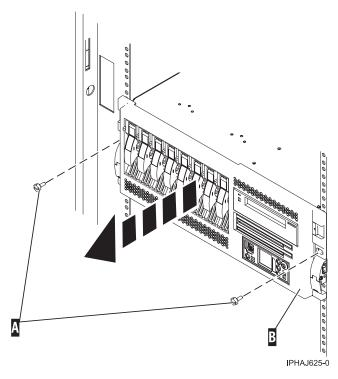
3. Release the rack latches A on both the left and right sides as shown in the following figure.
