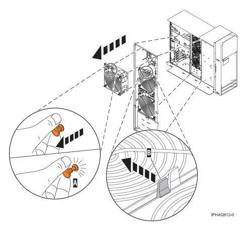
Figure 23. Removing the model 52x or, IntelliStation POWER 285 system unit fan unit in a stand-alone system
