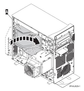
Figure 5. Replacing the model 7047-185 or 7037-A50 system unit air baffle in a stand alone system unit.
