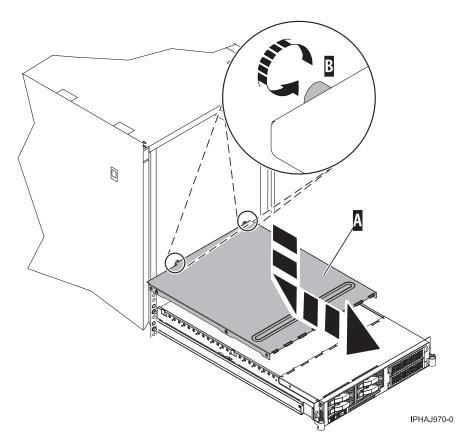
Figure 45. Install the service access cover on the rack-mounted model
