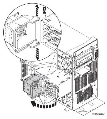
Figure 12. Removing the drive cage fan
