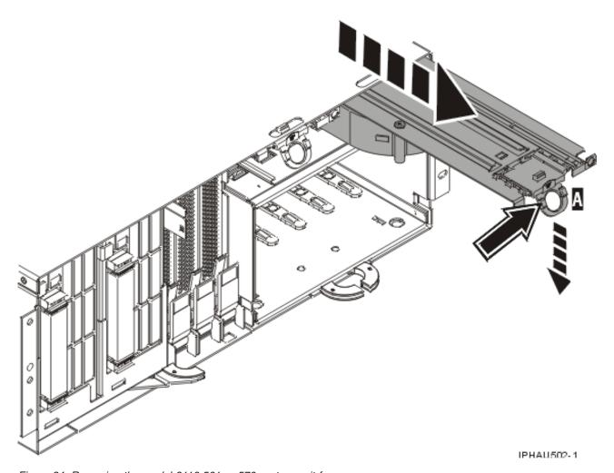
Figure 34. Removing the model 9116-561 or 570 system unit fan
