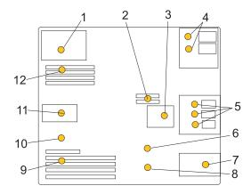
Figure 53. Light path diagnostic card indicator LED layout
