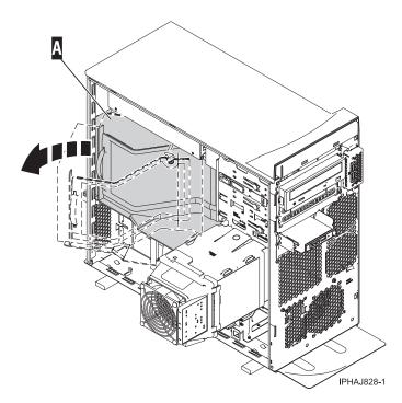
Figure 4. Removing the system unit air baffle in a stand-alone system
