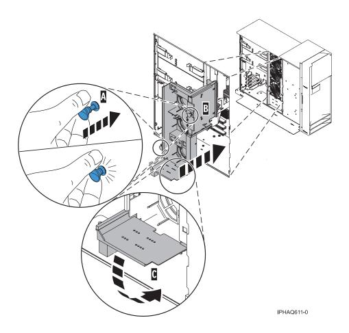
Figure 29. Replacing the fan tray assembly in a stand-alone system
