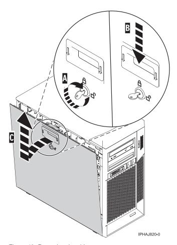
Figure 49. Removing the side cover
