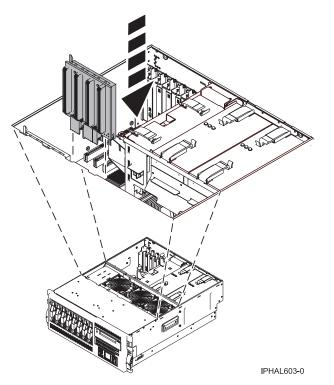
Figure 109. Replacing a disk-drive backplane in a rack-mounted system unit
