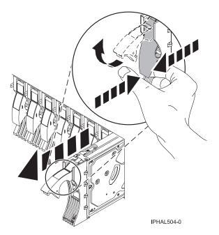
Figure 89. Removing a disk drive from a model 285, 52x, 55x, 9116-561, 570, 720, or 7311-D20
