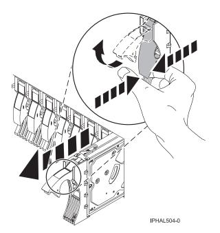
Figure 82. Removing a disk drive from a model 285, 52x, 55x, 9116-561, 570, 720, or 7311-D20
