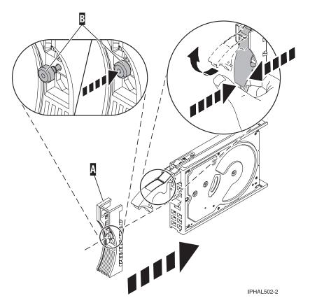
Figure 97. Attaching a disk-drive bezel
