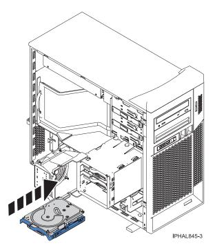
Figure 7. Installing the disk drive
