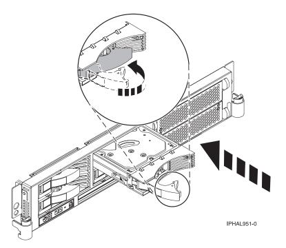
Figure 75. Installing a disk drive in a model 51x or 710
