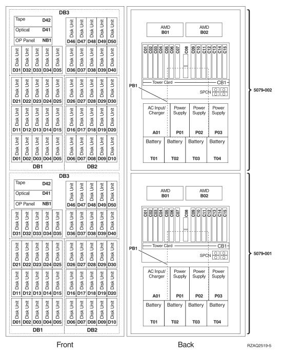
Figure 148. Disk drive locations for the 5294 and 8294 expansion unit
