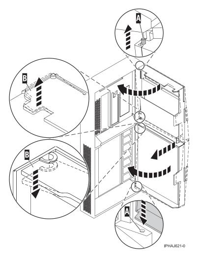
Figure 170. Installing the model 285 door
