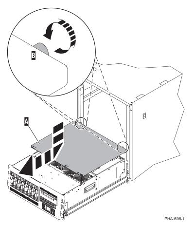
Figure 182. Install the service access cover on the rack-mounted model
