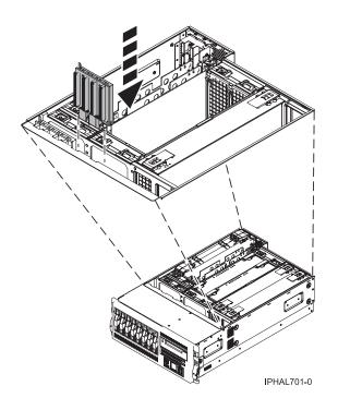
Figure 121. Replacing a disk-drive backplane in a rack-mounted system unit
