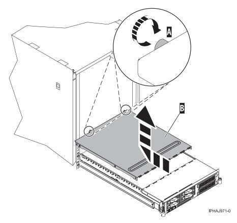
Figure 181. Remove the service access cover
