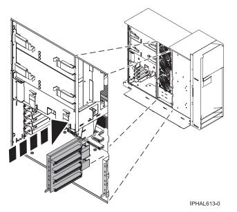
Figure 110. Replacing a disk-drive backplane in a stand-alone system unit
