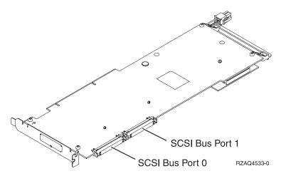
Figure 104. PCI adapter
