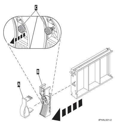
Figure 25. Removing a disk-drive bezel
