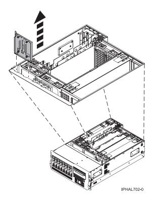
Figure 112. Removing a disk-drive backplane filler from a rack-mounted system unit
