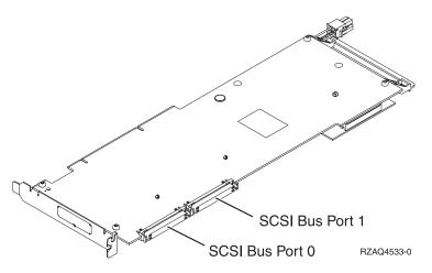
Figure 116. PCI adapter
