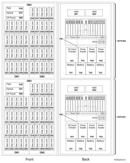
Figure 147. Disk drive locations for the 5079 expansion unit
