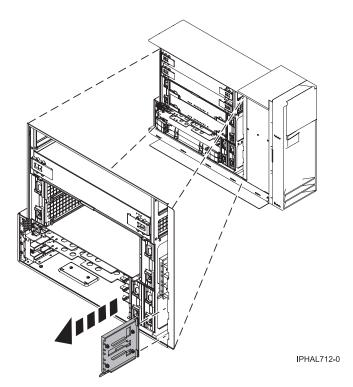
Figure 113. Removing a disk-drive backplane filler from a stand-alone system unit
