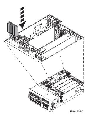
Figure 114. Installing a disk-drive backplane in a rack-mounted system unit
