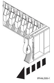
Figure 30. Removing a disk-drive filler from model 285, 52x, 9116-561, 570, 720, or 7311-D20
