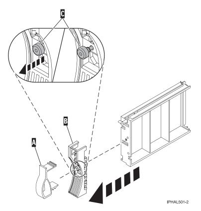
Figure 31. Removing the disk-drive bezel
