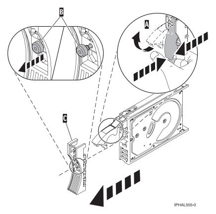
Figure 61. Removing a disk-drive bezel
