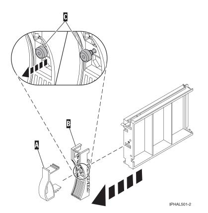
Figure 40. Removing a disk-drive bezel from the disk drive.
