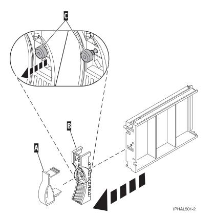
Figure 47. Removing a disk-drive bezel
