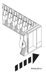
Figure 137. Installing a disk-drive filler
