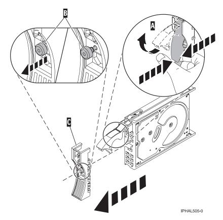
Figure 83. Removing a disk-drive bezel
