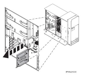
Figure 101. Removing a disk-drive backplane filler from stand-alone system unit
