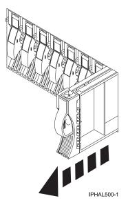
Figure 46. Removing a disk-drive filler from a model 285, 52x, 55x, 9116-561, or 570
