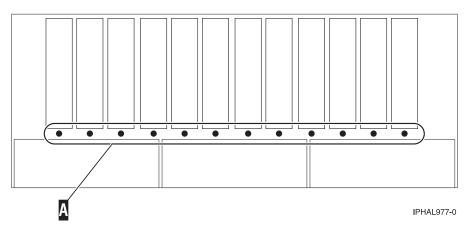
Figure 161. Front view of model 5786, 5787, 7031-D24 or 7031-T24 SCSI disk-drive enclosure concurrent maintenance lights
