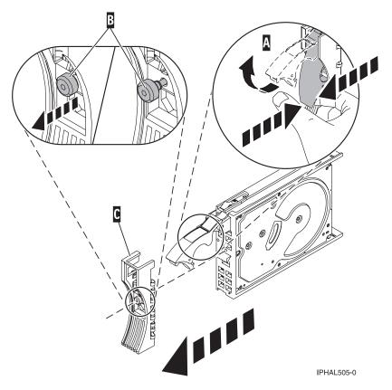
Figure 54. Removing a disk-drive bezel
