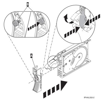
Figure 41. Attaching the disk-drive bezel to the disk drive.
