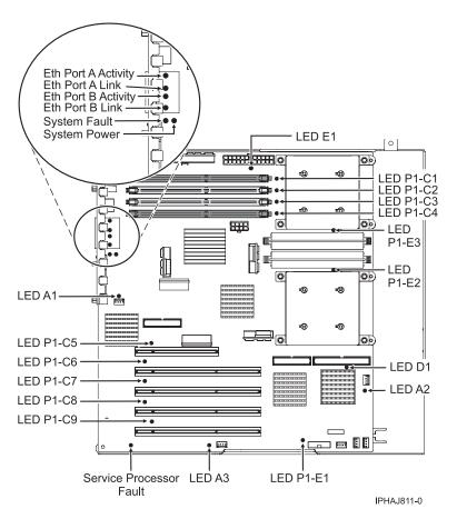
Figure 185. System backplane indicator LED layout
