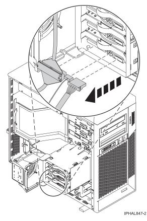
Figure 3. Unplugging cables from the disk drive
