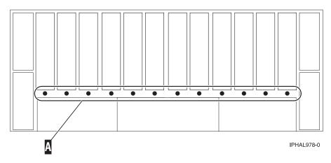
Figure 162. Back view of model 5786, 5787, 7031-D24 or 7031-T24 SCSI disk-drive enclosure SCSI disk-drive enclosure concurrent maintenance lights
