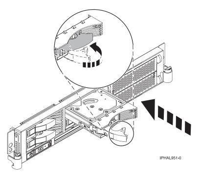
Figure 98. Installing a disk drive in a model 51x or 710
