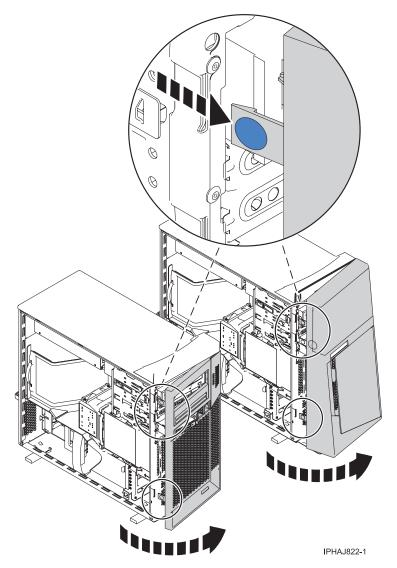
Figure 174. Removing the front cover
