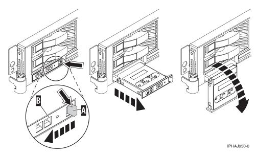
Figure 167. Gain access to the control panels
