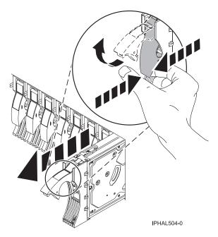
Figure 13. Removing a disk drive
