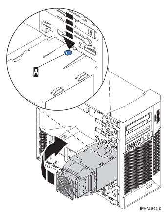
Figure 10. Rotating the drive cage into the system
