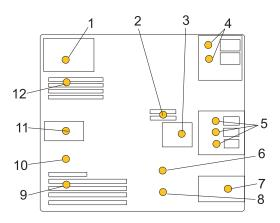
Figure 184. Light path diagnostic card indicator LED layout
