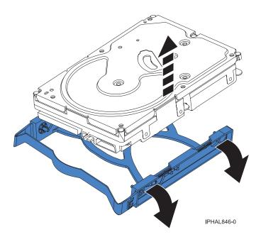
Figure 5. Removing the disk drive from the drive tray
