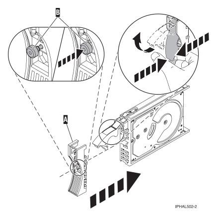
Figure 32. Installing a disk-drive bezel
