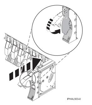
Figure 50. Installing a disk drive in a model 285, 52x, 55x, 9116-561, 570, 720, or 7311-D20
