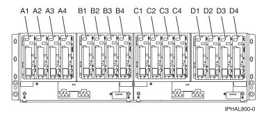
Figure 149. Disk drive locations for the 5791 and 7040-61D expansion units
