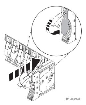
Figure 111. Installing a disk drive
