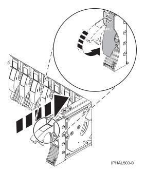
Figure 123. Installing a disk drive
