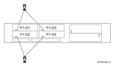
Figure 157. Model 51x and 710 disk-drive concurrent maintenance lights
