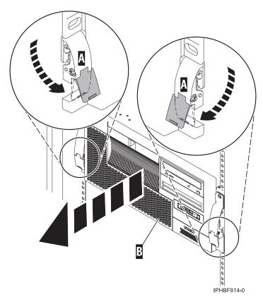
Figure 179. Placing the model in the service position
