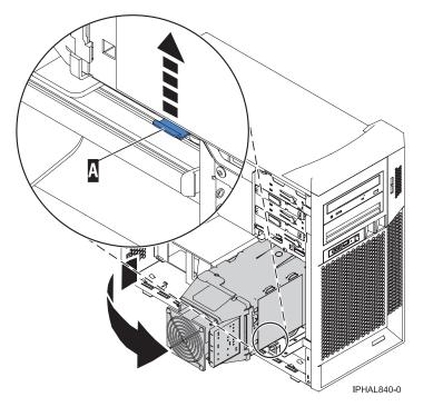
Figure 1. Rotating the drive cage out of the system
