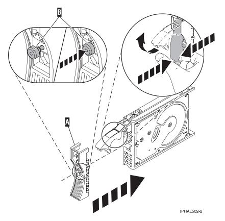
Figure 72. Attaching a bezel to the disk drive
