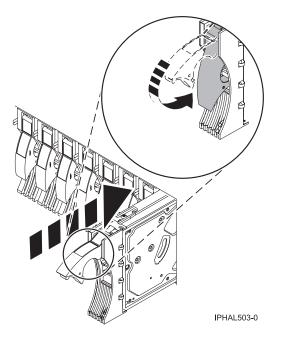
Figure 87. Installing a disk drive in a model 285, 52x, 55x, 9116-561, 570, 720, or 7311-D20
