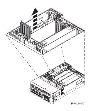
Figure 119. Removing a disk-drive backplane from a rack-mounted system unit
