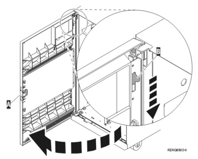
Figure 171. Removing the expansion unit front door
