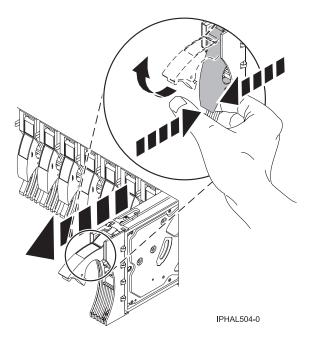
Figure 70. Removing a disk drive from a model 285, 52x, 55x, 9116-561, 570, 720, or 7311-D20
