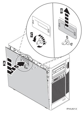
Figure 178. Replacing the service panel
