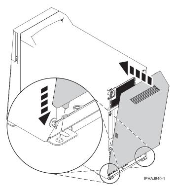
Figure 176. Replacing the back cover
