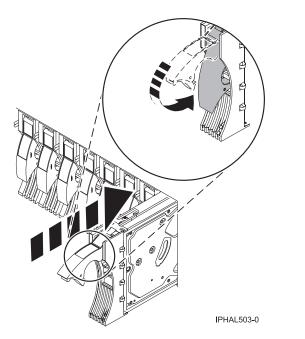
Figure 43. Installing a disk drive in a model 285, 52x, 55x, 9116-561, 570, 720, or 7311-D20
