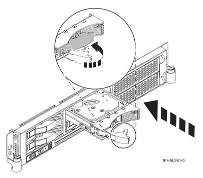
Figure 86. Installing a disk drive in a model 51x or 710
