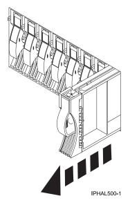
Figure 106. Disconnecting a disk-drive filler
