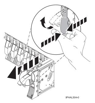
Figure 105. Disconnecting a disk drive from the disk-drive backplane
