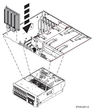
Figure 102. Installing a disk-drive backplane in a rack-mounted system unit
