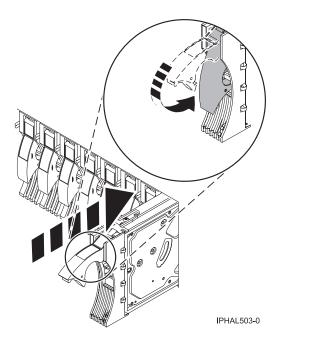
Figure 57. Installing a disk drive in a model 285, 52x, 55x, 9116-561, 570, 720, or 7311-D20
