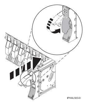
Figure 16. Installing a disk drive
