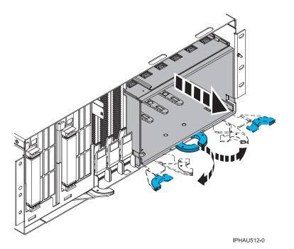
Figure 124. Removing a disk-drive enclosure
