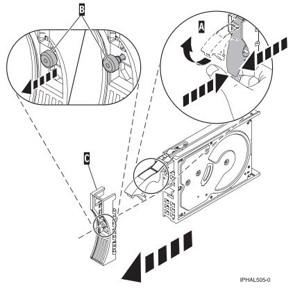
Figure 71. Removing a disk-drive bezel
