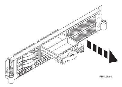
Figure 133. Removing a disk-drive filler from a model 51x or 710
