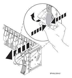
Figure 60. Removing a disk drive
