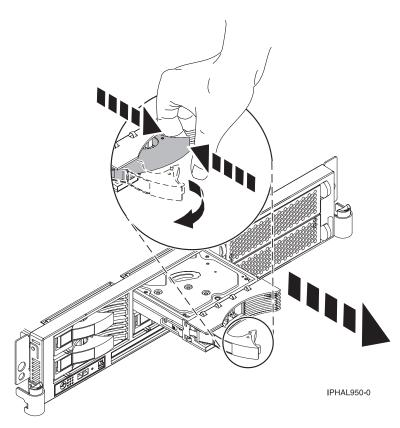
Figure 69. Removing a disk drive from a model 51x or 710
