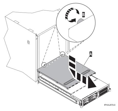
Figure 183. Install the service access cover on the rack-mounted model
