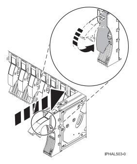
Figure 63. Installing a disk drive
