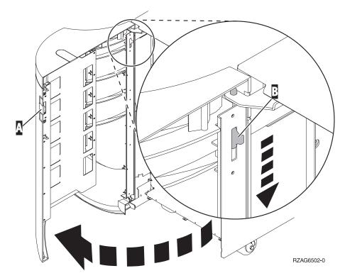
Figure 173. Removing the expansion unit back door
