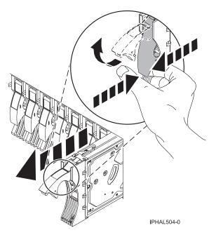
Figure 95. Removing a disk drive from a model 285, 52x, 55x, 9116-561, 570, 720, or 7311-D20
