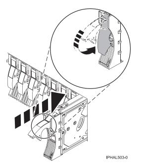
Figure 99. Installing a disk drive in a model a model 285, 52x, 55x, 9116-561, 570, 720, or 7311-D20
