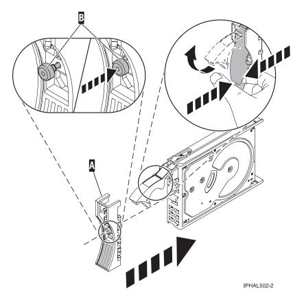
Figure 84. Attaching a bezel to the disk drive
