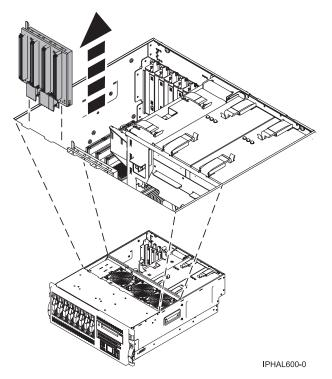
Figure 107. Removing a disk-drive backplane from rack-mounted system unit
