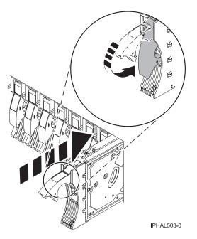
Figure 132. Installing a disk drive
