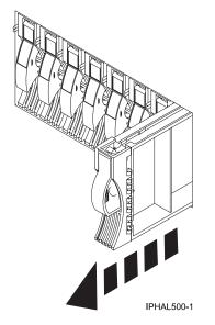
Figure 18. Removing a disk-drive filler from a model .285, 52x, 55x, 9116-561, 570, 720, or 7311-D20
