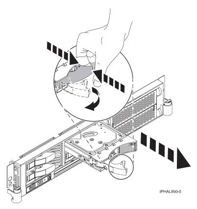
Figure 88. Removing a disk drive from a model 51x or 710
