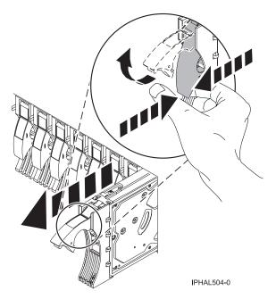
Figure 53. Removing a disk drive from a model 285, 52x, 55x, 9116-561, 570, 720, or 7311-D20
