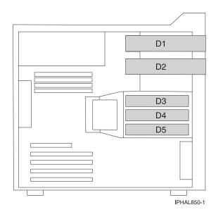
Figure 140. Model 7037-A50 and 7047-185 disk drive locations
