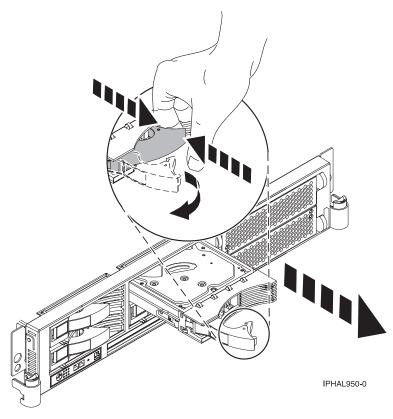
Figure 94. Removing a disk drive from a model 51x or 710
