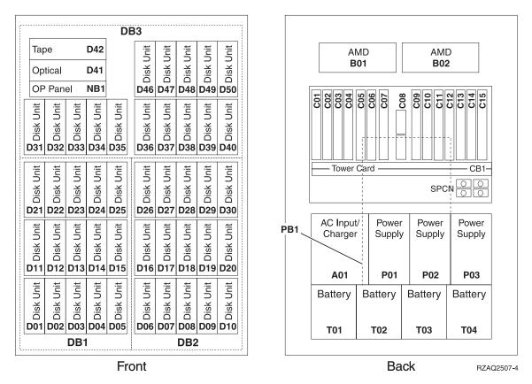
Figure 144. Disk drive locations for the 5074 expansion unit
