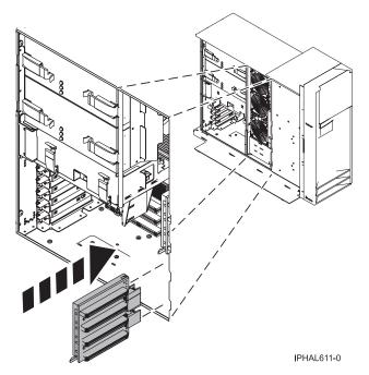
Figure 103. Installing a disk-drive backplane in a stand-alone system unit
