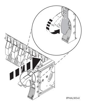
Figure 93. Installing a disk drive in a model 285, 52x, 55x, 9116-561, 570, 720, or 7311-D20
