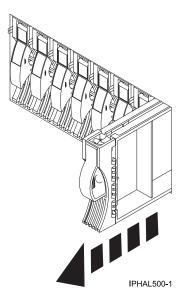
Figure 39. Removing a disk-drive filler from model 285, 52x, 55x, 9116-561, 570, 720, or 7311-D20
