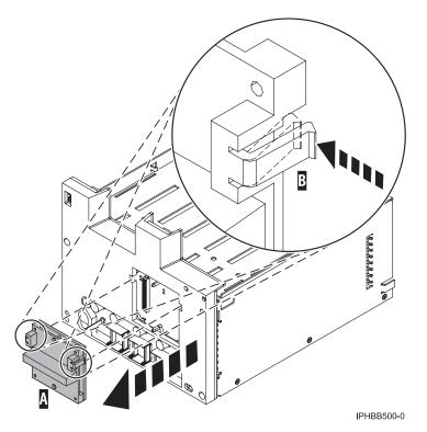
Figure 129. Removing a SCSI-IDE converter card
