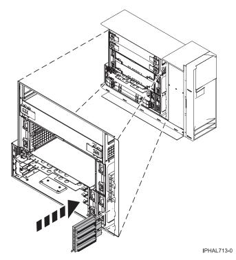
Figure 115. Installing a disk-drive backplane in a stand-alone system unit
