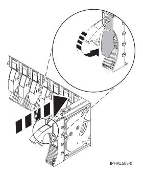
Figure 28. Sliding the disk drive in to the system unit
