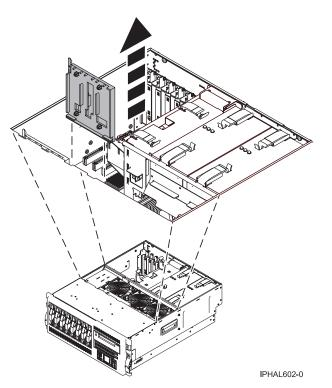
Figure 100. Removing a disk-drive backplane filler from rack-mounted system unit
