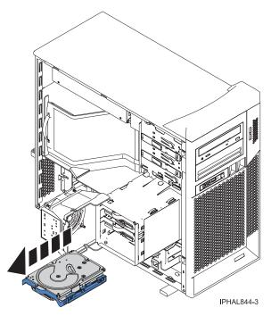
Figure 4. Removing the drive tray
