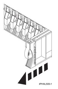
Figure 24. Removing a disk-drive filler
