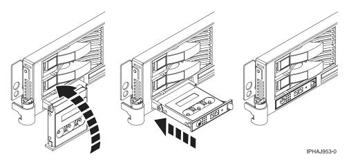
Figure 168. Close the control panels
