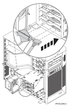
Figure 8. Plugging the cables in to the disk drive
