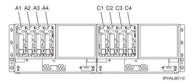
Figure 150. Disk drive locations for the 5794 expansion unit
