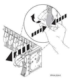
Figure 51. Removing a disk drive
