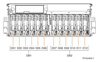
Figure 151. Disk drive locations for the 7311-D20 expansion unit
