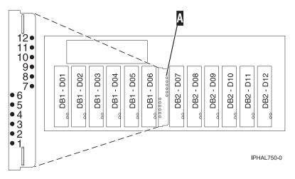
Figure 160. Model 7311-D20 disk-drive concurrent maintenance lights
