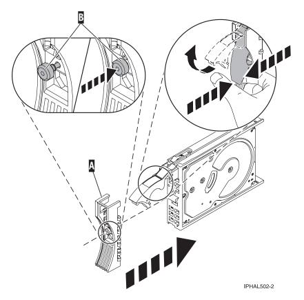
Figure 48. Installing a disk-drive bezel
