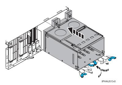
Figure 131. Installing a disk-drive enclosure
