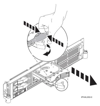
Figure 52. Removing a disk drive from a model 51x or 710
