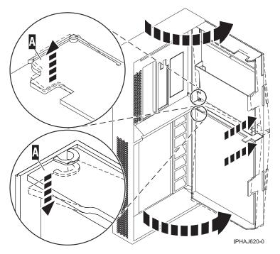
Figure 169. Removing the model 285 or 9131-52A door
