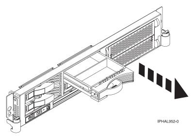
Figure 29. Removing a disk-drive filler from model 51x or 710
