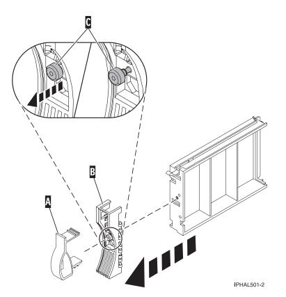
Figure 135. Removing a disk-drive bezel
