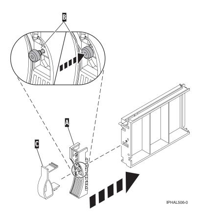
Figure 136. Attaching a bezel to a disk-drive filler
