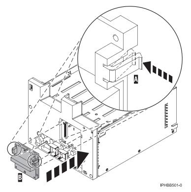
Figure 126. Installing a SCSI-IDE converter card
