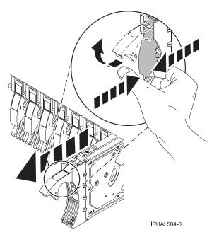
Figure 117. Disconnecting a disk drive from the disk-drive backplane
