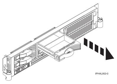
Figure 17. Removing a disk-drive filler from a model 51x or 710
