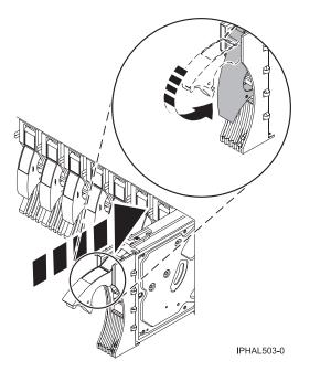
Figure 22. Installing a disk drive in a model 285, 52x, 55x, 9116-561, 570, 720, or 7311-D20
