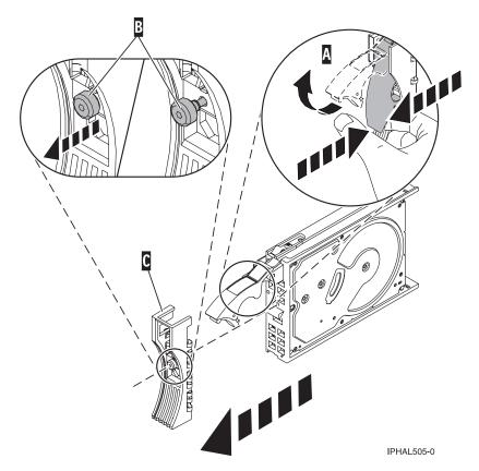
Figure 90. Removing a disk-drive bezel
