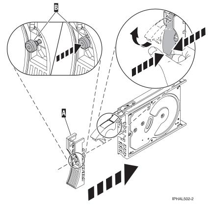
Figure 62. Installing a disk-drive bezel
