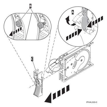
Figure 14. Removing a disk-drive bezel
