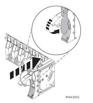
Figure 34. Installing a disk drive in a model 285, 52x, 55x, 9116-561, 570, 720, or 7311-D20
