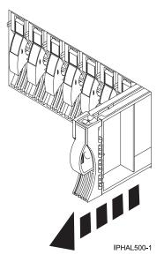
Figure 118. Disconnecting a disk-drive filler
