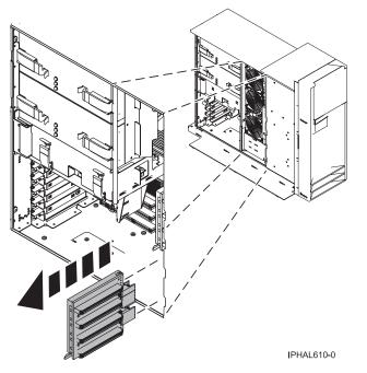
Figure 108. Removing a disk-drive backplane from stand-alone system unit
