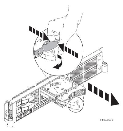
Figure 81. Removing a disk drive from a model 51x or 710
