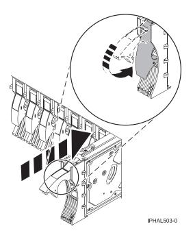
Figure 128. Installing a disk drive
