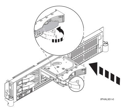
Figure 33. Installing a disk drive in model 51x and 710
