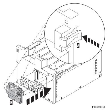
Figure 130. Replacing a SCSI-IDE converter card
