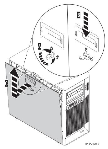
Figure 177. Removing the side cover
