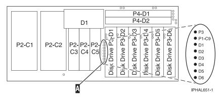
Figure 158. Model 9116-561 or 570 disk-drive concurrent maintenance lights
