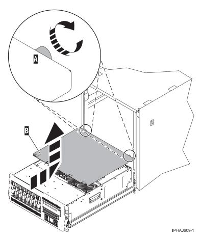
Figure 180. Remove the service access cover
