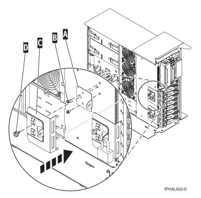
Figure 154. Installing a locking device on stand-alone system
