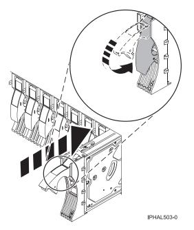
Figure 76. Installing a disk drive in a model 285, 52x, 55x, 9116-561, 570, 720, or 7311-D20
