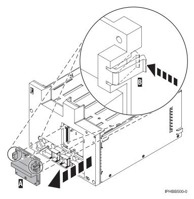
Figure 125. Remove a SCSI-IDE converter card
