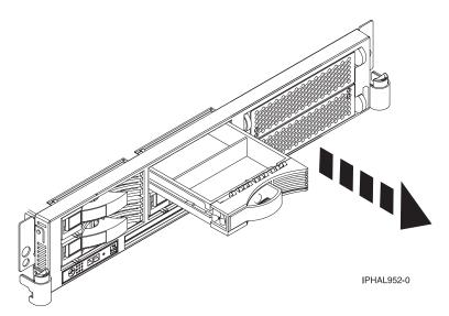
Figure 38. Removing a disk-drive filler from model 51x and 710
