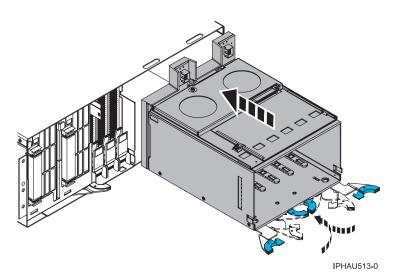
Figure 127. Replacing a disk-drive enclosure
