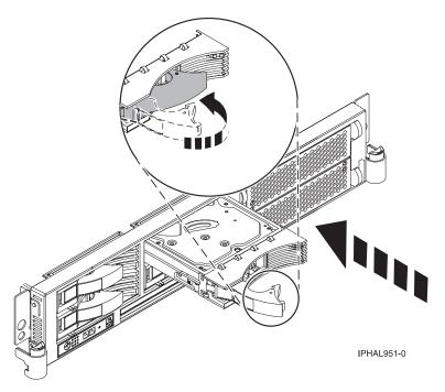
Figure 49. Installing a disk drive in a model 51x or 710
