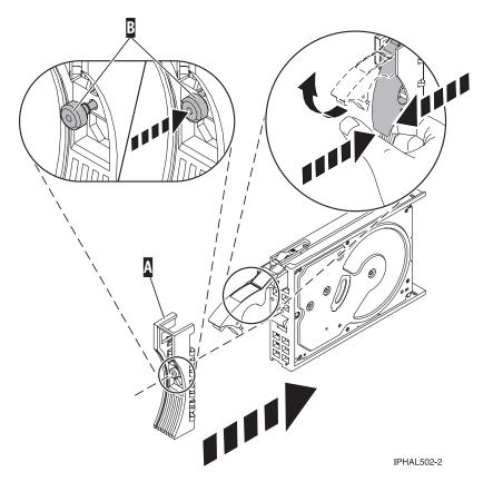
Figure 15. Installing a disk-drive bezel
