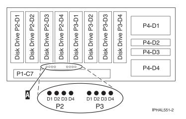
Figure 156. Model 285, 52x, 55x, and 720 disk-drive concurrent maintenance lights
