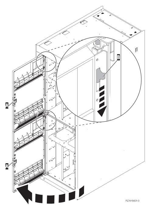
Figure 172. Removing the expansion unit front door
